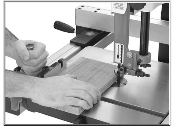
Figure 43. Making a 90° crosscut.
